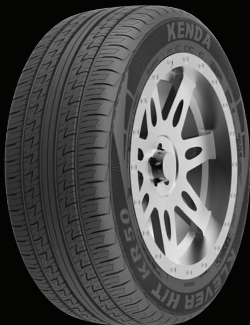
Four wide circumferential grooves and extreme siping help maintain wet traction and braking performance. Solid center rib provides great fuel economy and excellent handling capability. Random variable pitch tread arrangement provides great wear, low noise, and smooth ride.
