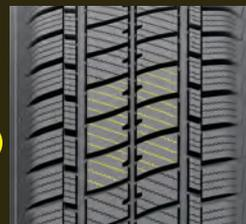
Zigzag 3D sipes for enhanced snow traction capabilities with considerable interlocking for wet and dry braking.
