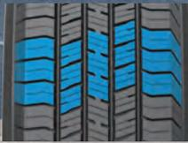
Computer-optimized footprint for excellent wear and handling under multiple load conditions.
