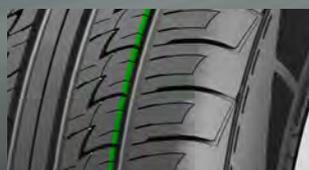
Straight groove edge chamfering design increases stability during cornering.
