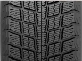
Unidirectional tread design for snow maximum traction.
