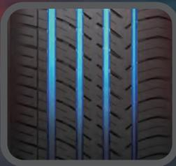
Four large circumferential grooves provide great hydroplaning and wet traction performance.
