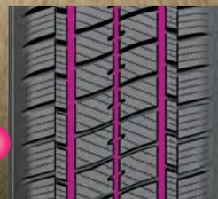
3 see-through longitudinal grooves improve water drainage, maximizing overall wet performances and handling on snow surfaces.
