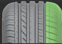
Low void outside tread portion maximizes dry handling, traction performance, and cornering stability.
