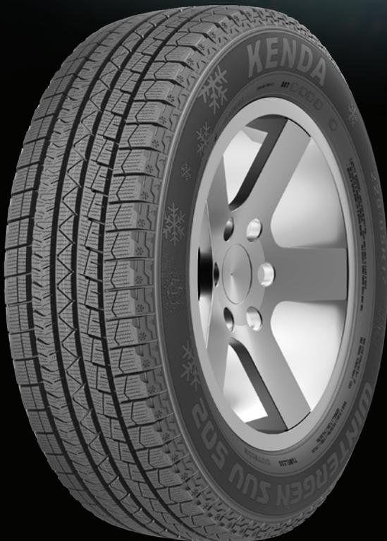
Hundreds of zigzag sipes coupled with an enhanced chemical rubber compound provides confident, reliable grip in icy and snowy conditions. The drainage grooves increase water clearance efficiency, while the square tire shoulder design reduces braking distance.
