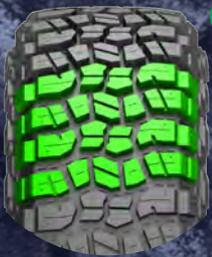
● Interlocking tread pattern for optimized off-road forward and later traction
