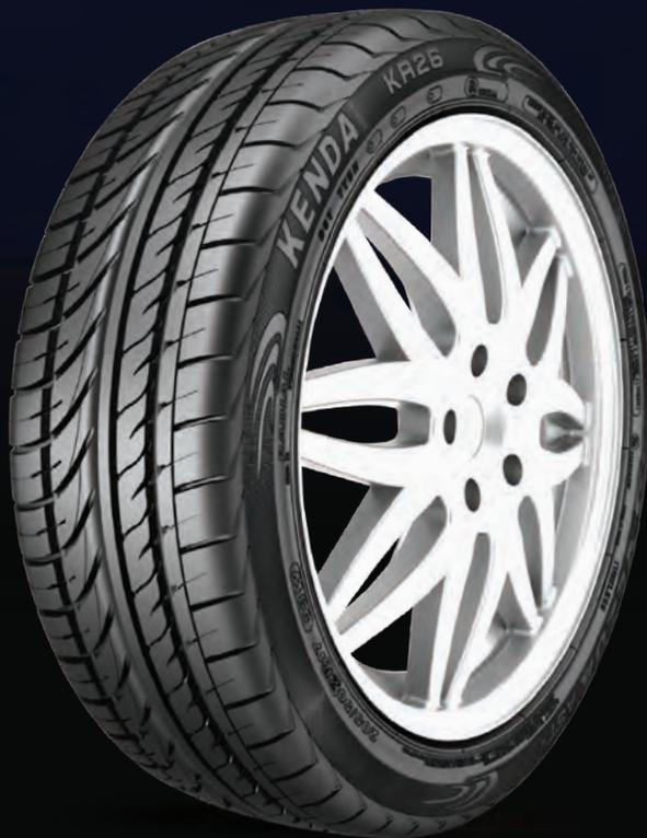
The KR26 VEZDA AST is KENDA's high performance sport tire with a range of 14~17 inch sizes and H, V and W rated tires. The asymmetrical tread design provides excellent durability, handling, and cornering. The five-pitch sequence tread design offers a quiet, comfortable ride, while the four wide circumferential grooves provide outstanding handling and cornering stability. The inside shoulder with a high void ratio design evacuates water for excellent wet performance.
