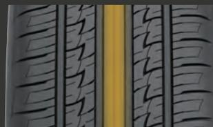
Straight-line stability is improved by the center block placement.
