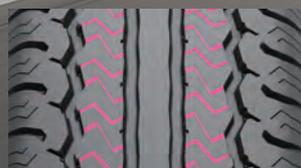
Lightning-shaped pattern design on the center tread increases drainage and safety on wet surfaces.
