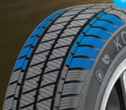
Shifted slot in the shoulder area reduces noise and enhances lateral snow performance. Its design allows to rebalance the block stiffness enhancing the wear performance.
