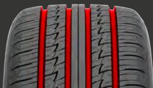
Four main grooves improve drainage and wet braking performance.
