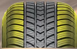
Both sides efficiently exclude water and snow and provide driving stability.
