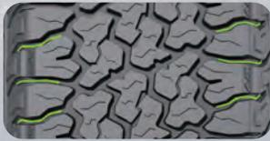
Stone ejectors effectively remove rocks and mud from the pattern.
