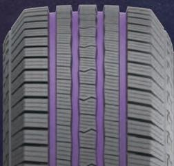
● Four large circumferential grooves provide superior hydroplaning/wet traction performance.
