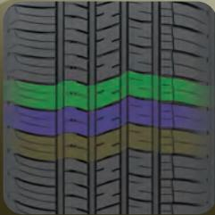
■ Computer-optimized pitch sequencing provides excellent noise and wear performance.
