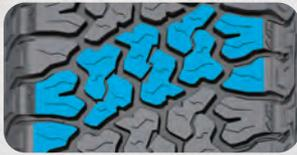
The high-stiffness and multi-angle blocks design to get extraordinary grip performance and resist the damage of pattern blocks in harsh road conditions.
