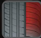
Outside wide and high rigidity block design enhance cornering stability and traction.
