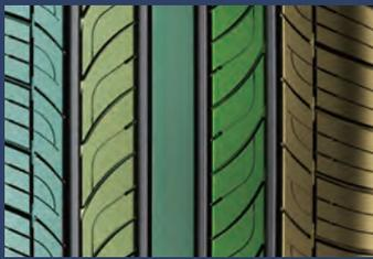
Wider shoulder siping and circumferential grooves help to displace water for ultimate traction in wet or dry conditions.
